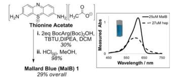
**Figure 2.** Synthetic scheme for new dye mallard blue (MalB, 1) along with the UV–visible absorption band at 615 nm ( $25 \,\mu$ M, photo) before (solid line) and after (dashed line) binding to heparin.
