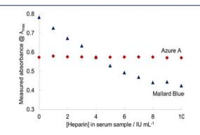
**Figure 7.** Graph showing measured UV absorbance at  $\lambda_{max}$  for mallard blue ( $\lambda_{max}$  615 nm) and azure A ( $\lambda_{max}$  634 nm) upon titration of heparin-containing serum.
