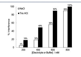
**Figure 4.** Extent to which electrolyte (open bars) or buffer (filled bars) disrupts the MalB-heparin interaction compared to binding in pure water as quantified by the absorption from UV–vis spectroscopy at 615 nm.
